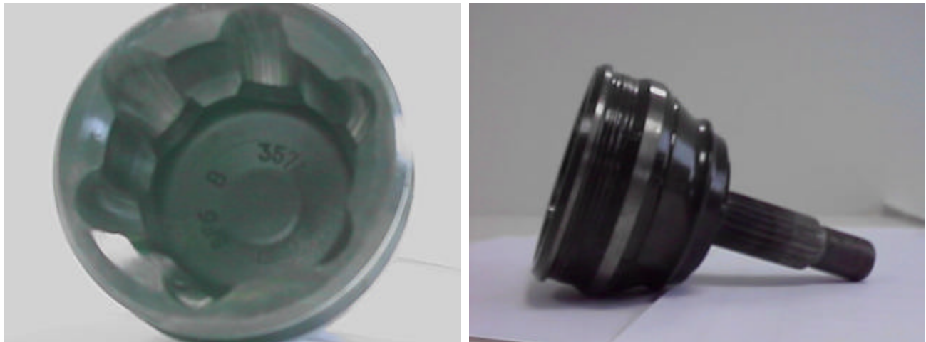
Figure 1 Pictures of a typical CV constant velocity joint
